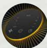
Air quality sensor: green light: good; orange light: medium; red light: bad
